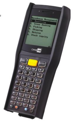
Wireless capabilities give easy access to peripherals and servers, keeping workers in-touch and always a step ahead of the task at hand. The largestin-class backlit, 2.6-inch, 160x160 pixel display makes work simple, even in dark corners. Drops, humidity, or freezing temperatures won't stop the CipherLab 8470 mobile computer. It's built tough to work on the edge.
