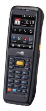
The 9200 series operates on a 3300 mAh battery which minimizes the need to change batteries and allows easy data capturing for extended time. With long lasting power, it also supports versatile reader options in linear imager, laser, 2D imager, and RFID to effectively assist you with different scanning needs.
