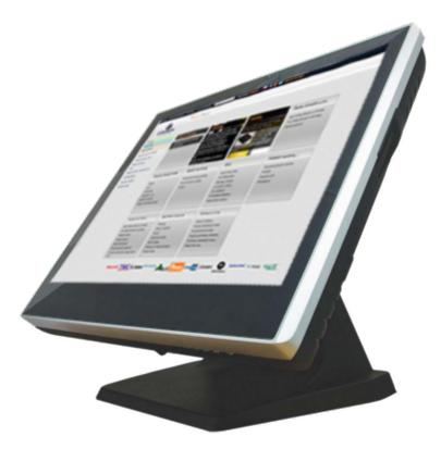
Models with technology tFLAT have no protruding edges around the touchpad, allowing the seamless touch-screen and in the regions. This makes them even more resistant eg. Against liquid spills and their maintenance is much easier.
