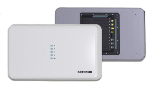
The core function of the ARU 8500 is a circular switch-beam antenna. In contrast to standard RFID antennas, the antenna beam here can be swivelled in three areas to track the direction of movement in a gantry or when the goods pass through a gate. The otherwise easily detected pass-through area is divided into three zones in order to reliably determine the direction of movement when the goods pass through the gate (zone 1 to 3; zone 3 to 1).
