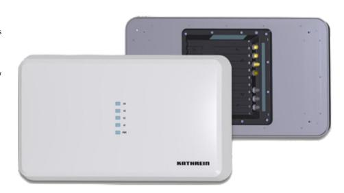
The core function of the ARU 8500 is a circular switch-beam antenna. In contrast to standard RFID antennas, the antenna beam here can be swivelled in three areas to track the direction of movement in a gantry or when the goods pass through a gate. The otherwise easily detected pass-through area is divided into three zones in order to reliably determine the direction of movement when the goods pass through the gate (zone 1 to 3; zone 3 to 1).
