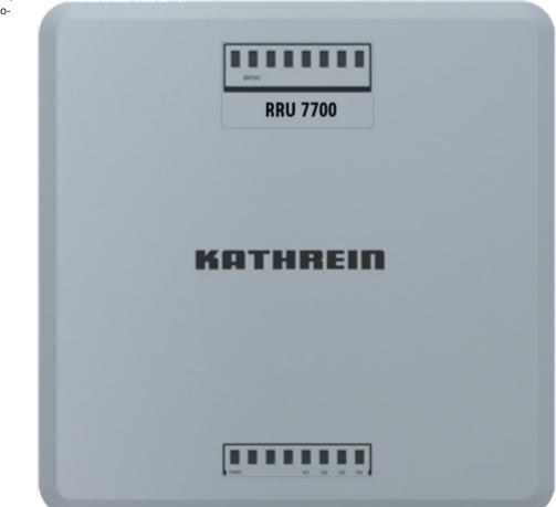
With its best-in-class +33 dBm UHF RFID unit and PoE+ powering capability, the reader is the first choice for vehicle identification in harsh environments. Based on the latest RFID standards, such as EPC Gen2v2/ISO 18000-63, Kathrein RRU 7700 reader supports all market-leading transponder chips for security, authentication and encoding. This makes the reader compliant to the Crypto Suite requirements for road tolling of ISO/IEC 29167-10.
