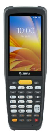
Zebra has equipped the MC2200 and MC2700 with a numeric keyboard with 34 keys. Great Care was taken to ensure that the size, shape and position of the keys are easy to use, even when wearing gloves. Thanks to the high-contrast colour, they are equally easy to see both during the day and at night. Furthermore, two additional finger rods ensure that the mobile computers may be operated comfortably with just one hand, yet held securely.
