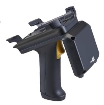
The RK25 UHF RFID reader complies with EPC Global Gen2 v2 standard and the RFID reader can read RFID tags in common supply chain. The Gen2 v2 standard can satisfy higher security and privacy requirements, which is ideal for applications such as retail and healthcare. The RS35 UHF RFID reader has the high-speed ability to read over 900 tags per second with a reading range of over 8 meters. It does more than satisfy the long-range reading demands of the warehouse/in-store inventory management.
