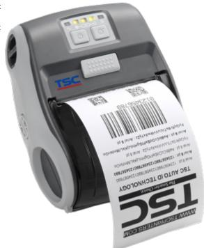
TSC printers have the <u>Thermal Smart Control technology</u>, a patented electronic print head temperature control. Print output is sharper because of that technology and, what's even more important, printhead life is several times longer.
